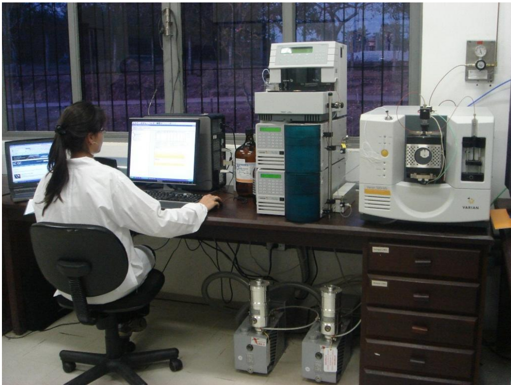
HPLC-MS facility at Bioprospecting Associated Laboratory
