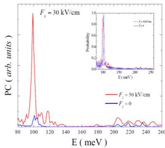
Figure 1 – Photocurrent response with and without the application of an electric field to the QDIP structure.
