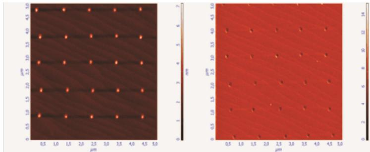
Figure 36 – Atomic force microscopy images of oxide dots (left) and the resulting pattern of depressions produced after the oxide is removed (right), on an InP surface.
