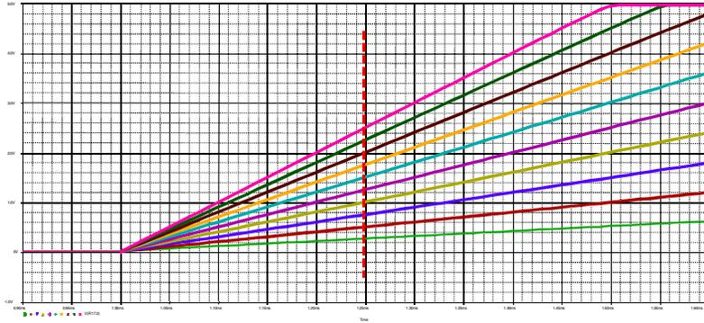
Figure 20. Output due to various photo-generated currents (10nA to 100nA in 10nA linear steps)
