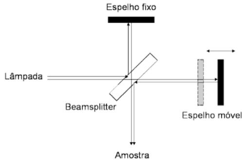
Figure 34 Experimental setup for measurement of the photocurrent with the FTIR spectrometer.
