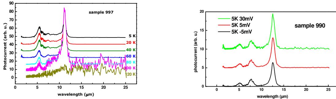
Figure 5 (a) Photocurrent as a function of temperature for another QDIP structure, showing the possibility of detecting radiation of two different wavelengths. (b) Photocurrent for a QDIP structure for three different applied bias showing the possibility of detecting radiation of three different wavelengths.
