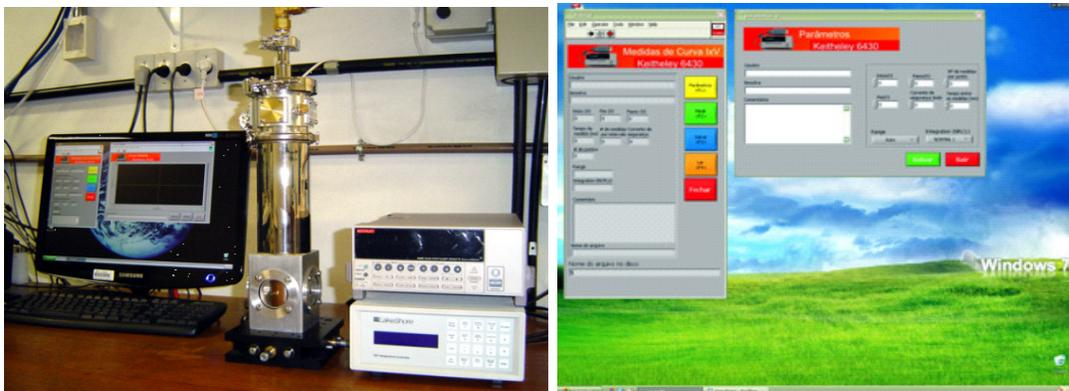
**Figure 12:** (Left) Full I-V curve system with 77 – 300 K capability. From left to right, we can see the monitor showing some windows of the control software, the optical cryostat, the source meter (above) and the temperature controller (below). (Right) Main menus of the control software running under Labview.
