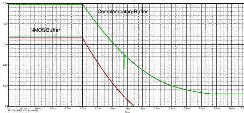
Figure 18. Comparison of the CAPS output signal with that of a conventional APS with NMOS.
