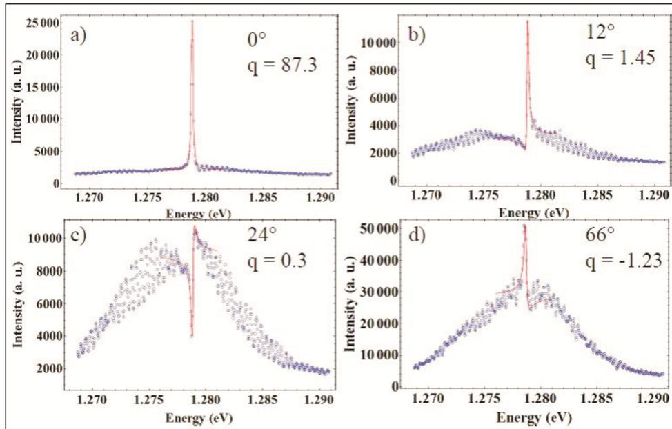
Figure 43 – Reflectivity spectra of a photonic crystal with a L3 cavity, for different polarization angles of the incoming light. The dots represent the experimental data and the red lines are fits considering a Fano interference between the photonic mode and the reflectivity continuous. The Fano parameter  $q$ , shown for each spectra, is the only adjustable parameter.
