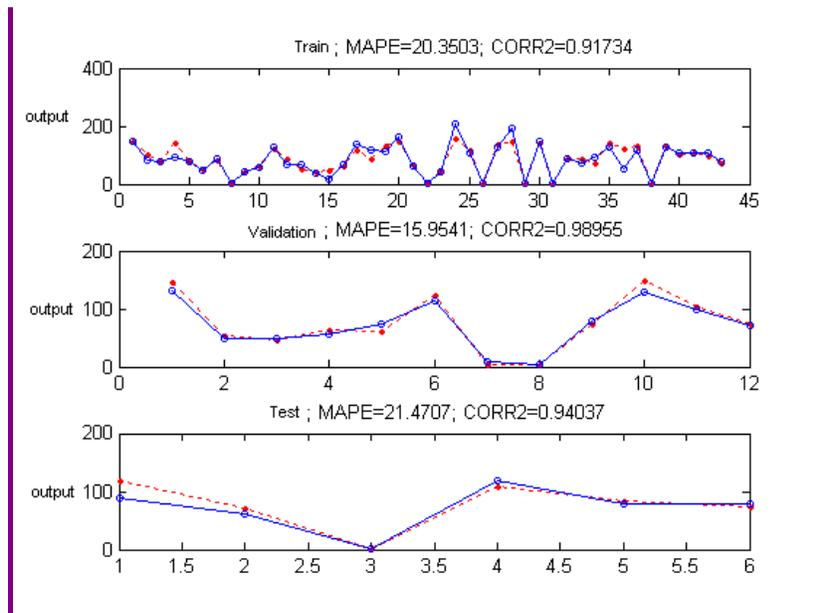
Figure 38 - Comparison of the prediction by neural networks for the density of quantum dots
