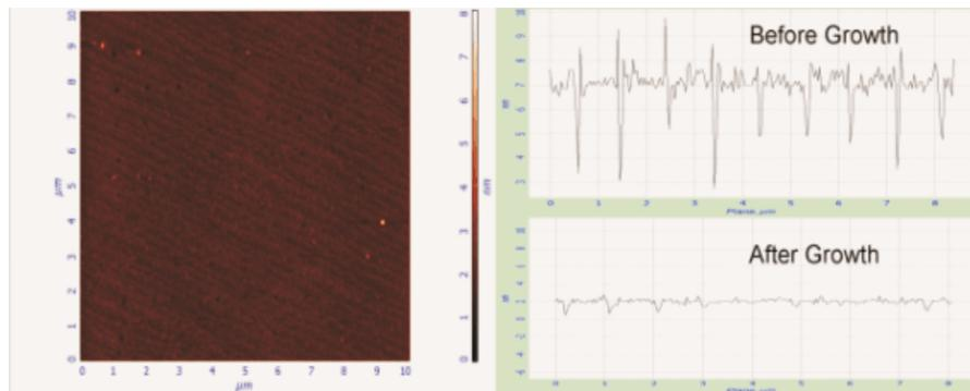
Figure 37 – The figure in the right is an image of atomic force microscopy of a InGaAs surface lattice matched with the InP substrate. The good quality of the surface demonstrates the quality of the growth. The diagrams in the left are height profiles obtained also by AFM before and after the InGaAs growth. The depressions are clearly seen before the InGaAs deposition. The profile obtained after growth shows that these depressions are nearly totally filled with InGaAs deposition.
