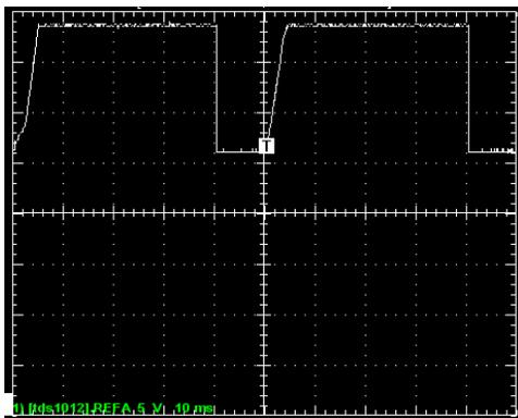
Figure 24 Signal CTIA output with bipolar reset switch.
