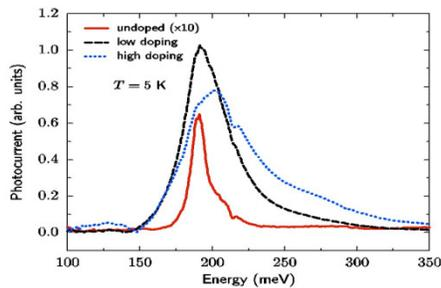
Figure 6 Photocurrent of a QDIP structure showing the change in the full width at half maximum of the peak with the doping level.
