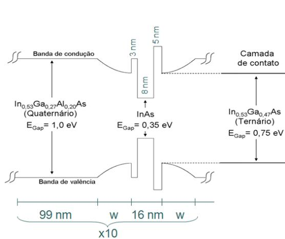
Figure 30 – Conduction band profile of the sample
