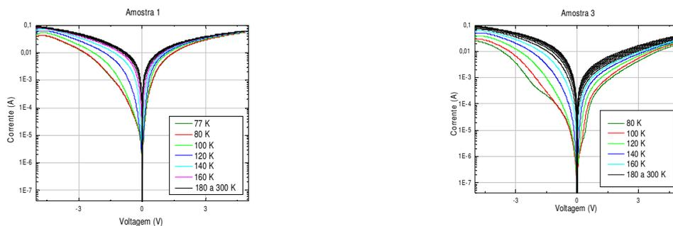
**Figure 14:**  $I \times V$  curves performed with the dark shield as a function of temperature for 2 QDIPs having a different Si doping of the contact layers: (left)  $10^{18} \text{ cm}^{-3}$ ; (right)  $5 \times 10^{17} \text{ cm}^{-3}$ .
