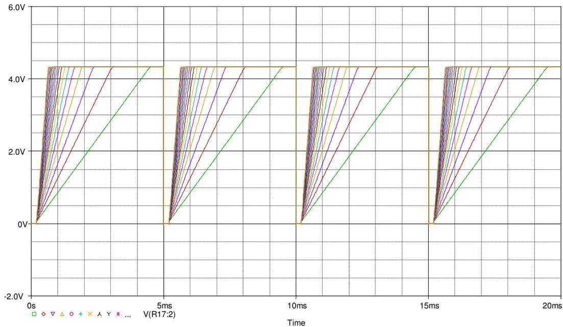
Figure 25. CTIA output with CD4066 reset switch
