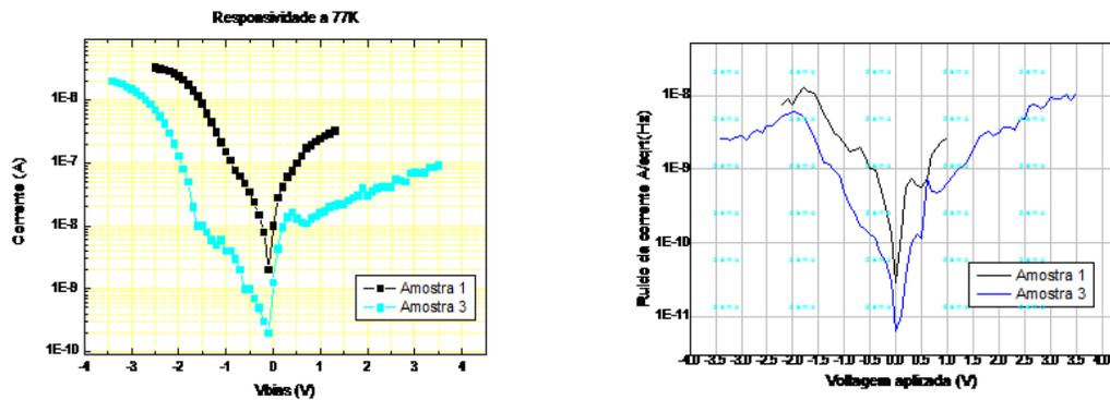
**Figure 15:** (esquerda) Responsivity curves (photocurrent) as a function of applied voltage for two QDIPs with different doping levels of the contact layers: (black)  $10^{18} \text{ cm}^{-3}$ ; (blue)  $5 \times 10^{17} \text{ cm}^{-3}$ . (right) Photocurrent noise measurements as a function of applied bias for the same two QDIPs.
