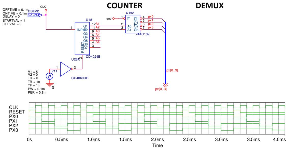
Figure 27 – Circuit for addressing pixels on an array and control-signal scheme.
