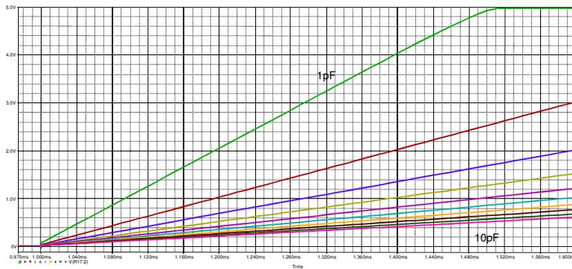
Figure 21. Output slope variation due to change in integrating capacitor value (1pF to 10pF in 1pF linear steps)
