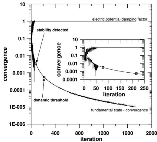
Figure 3 – A typical convergence curve obtained with the procedure adopted for self-consistent computation. The evolution of the dampin factor, the point where the stability is detected and the point where the iterative process is interrupted are also shown.
