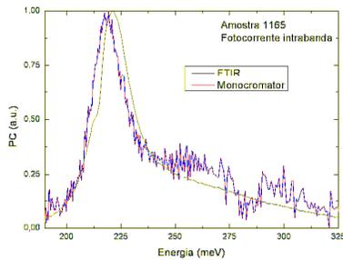
Figure 35 – Comparison of photocurrent response measurements from the FTIR and monochromator techniques.
