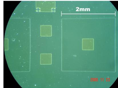
**Figure 11:** (Left) General QDIP structure, showing the active region (with 10 QDs layers) surrounded by two Si-doped layers that will receive the electrical contacts. (Right) Processed QDIP (after photolithography, wet etching and metal deposition), showing a 2mm x 2mm mesa with 0.5mm x 0.5mm top and bottom Ni/Ge/Au contacts.
