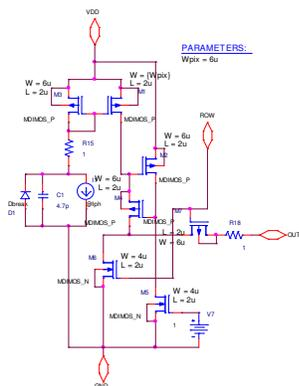
Figure 26 – Schematics of the current-mode pixel circuit.
