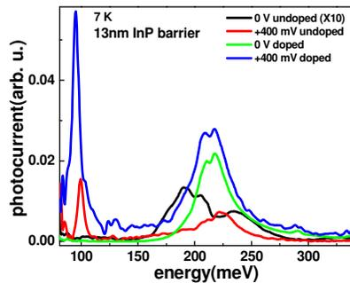
Figure 2- Photocurrent measured with and without applied electric field, in the same QDIP structure considered in the calculations.
