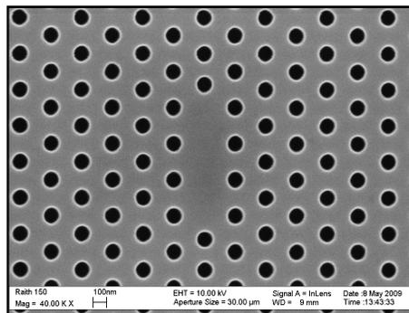
Figure 42 – Two dimensional photonic crystal, with a periodic triangular pattern of air holes in GaAs. The defect consists in the absence of three holes in line, the so-called L3 cavity.
