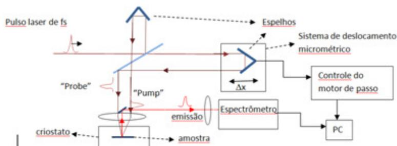
Figure 40 Experimental setup for pump & probe system, using a Ti:Sapphire laser pumped by a solid state CW laser.
