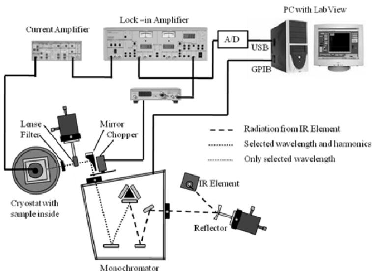
Figure 33 Setup for photocurrent measurements with a monochromator
