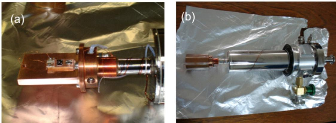
**Figure 13:** a) Sample fixed on the cold finger of the optical cryostat. b) Dark shield screwed around the sample in order to perform dark-current measurements. The dark shield and cold finger are in thermal contact with the liquid-nitrogen dewar that can be seen on the right.
