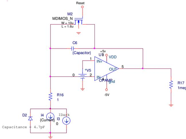
Figure 19. CTIA circuit schematics.
