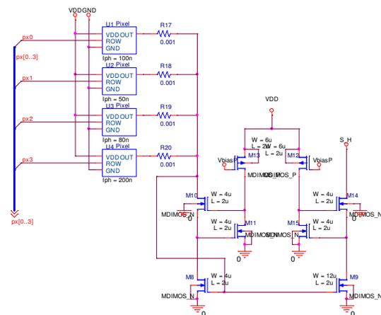
Figure 28 – Secondary current-mirror on a 4-pixel column bus.
