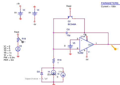
Figure 22. CTIA with bipolar reset switch.
