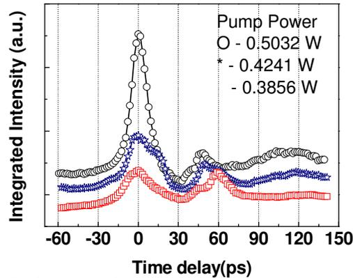
Figure 41: Emission intensity from polariton when excited by the pump and probe pulses as a function of delay and power intensity.
