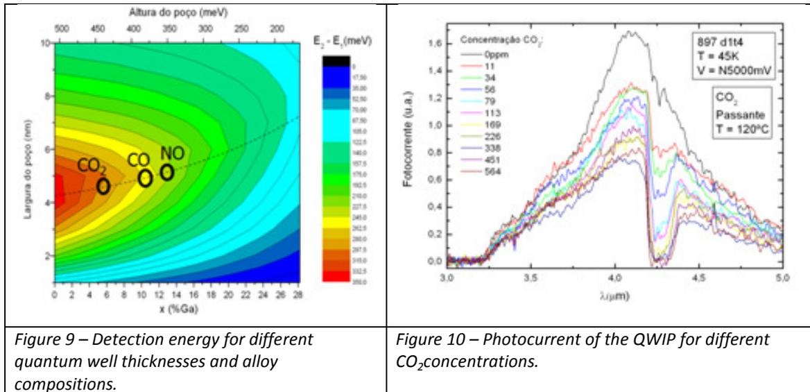
Figure 9 – Detection energy for different quantum well thicknesses and alloy compositions.
