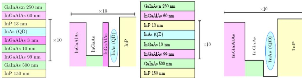
Figure 4 Scheme of QDIP structures for samples (a) 997 and (b) 990.
